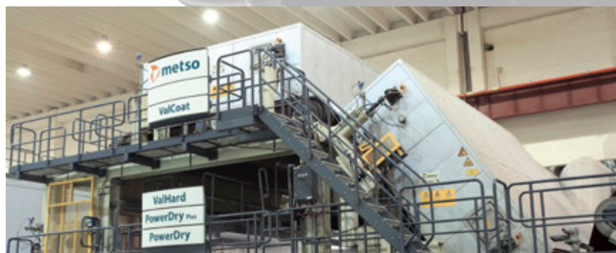
The coating drying uses PowerDry Plus gas drying instead of the conventional infrared drying.
