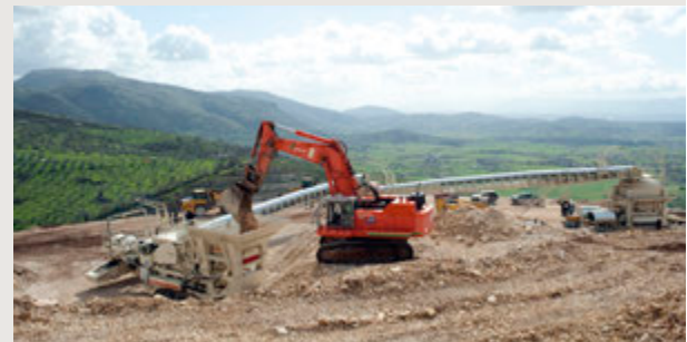
Metso's mobile primary crushing and conveying system consisting of Lokotrack LT140 jaw plant and Nordberg LL12 mobile conveyor feeds the crushed limestone to the stationary field conveyor.
