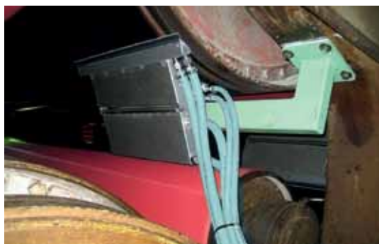
TailDoc tail threading units thread the sheet tail through the machine with the help of compressed air.
