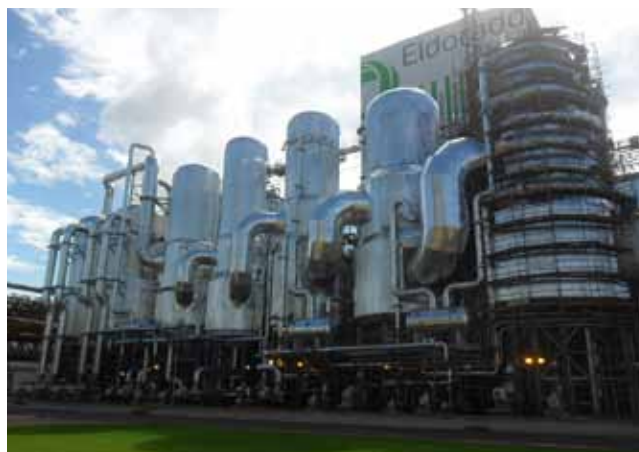
Metso-supplied evaporation plant and recovery boiler at Eldorado's Três Lagoas site.
