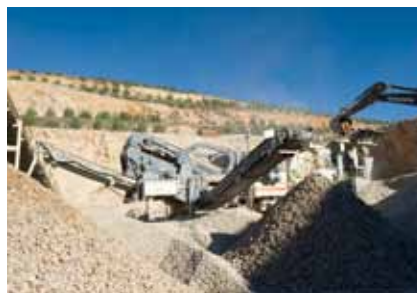
The Metso track-mounted crushing plants like LT1415S can be easily transported between the company's four quarries.
