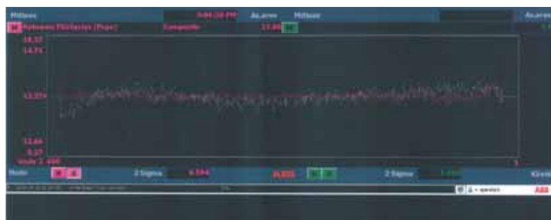
Coat weight profile measured at Stora Enso Anjala PM 2 by online scanner before (white) and after (purple) optimization. Profile skewness was eliminated and variation significantly reduced with iRoll Sizer.
