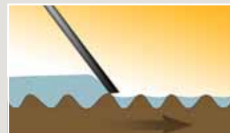
The first blade coating smooths the brown base board.
