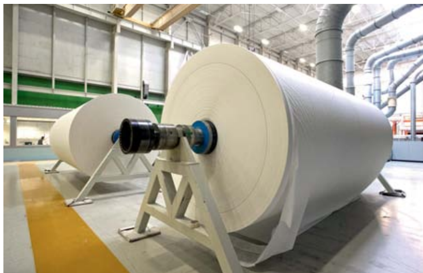
Excellent-quality jumbo rolls. The concept is mixed. Reeling on spools as well as split reel winding on cores.
