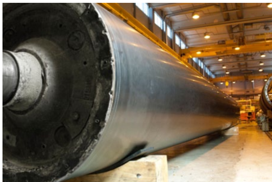
WireGem coating in excellent condition after 3-year run period at Propapier Burg PM 1.
