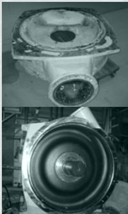
The new Turbine Housing increases refiner capacity by 30%.
